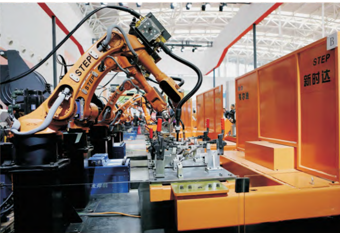
Frame assembly welding
