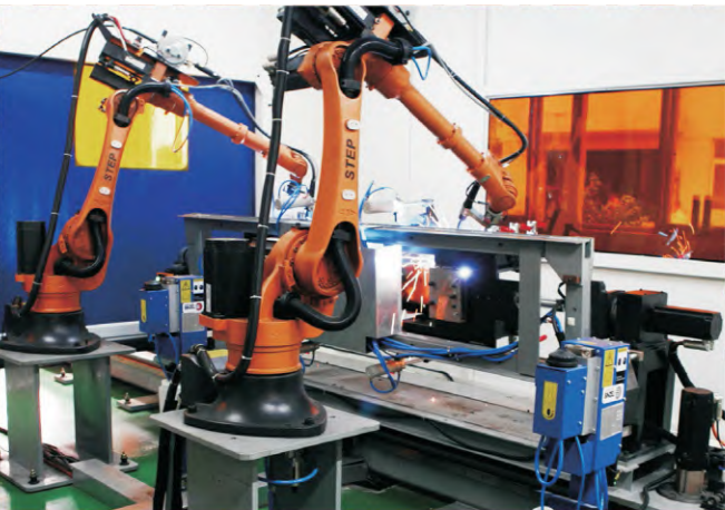
Elevator door panel reinforced hamstring welding
