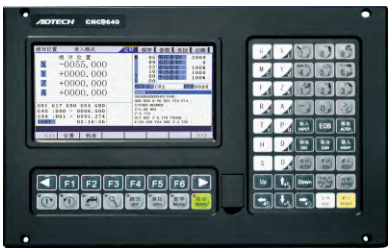
CNC9640 (4 axis) Popular 4 axis milling CNC controller
