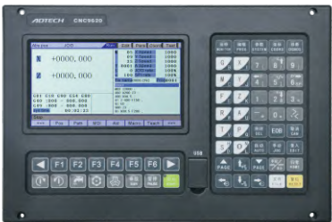
CNC 9620 (2 axis) Popular 2 axis lathe CNC controller
